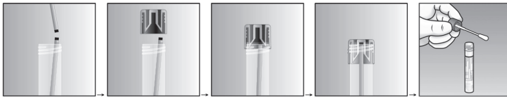
Fig 3. Capture of broken swab applicator stick by FecalSwab tube cap
